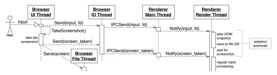
Fig. 2. Simplified view of how ChromePic processes user inputs that trigger a webshot. Dashed arrows indicate asynchronous calls.
