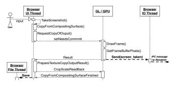
Fig. 3. Overview of how screenshots are taken and the Renderer is notified (notice that some of the function call names have been shortened and made more readable for presentation purposes, compared to the source code).
