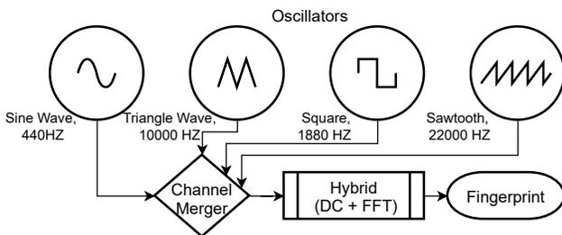
Figure 7: Merged Signals Method
